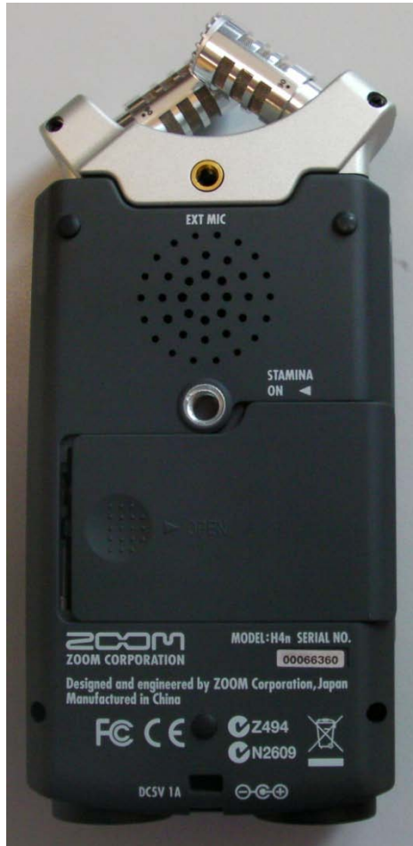
Figure 7 – Remove the battery cover by pressing down on the cover and sliding to the right.
