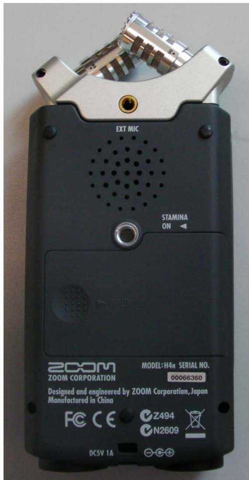
Figure 6 – Back of the Zoom recorder showing speaker, stand mount and battery cover.
