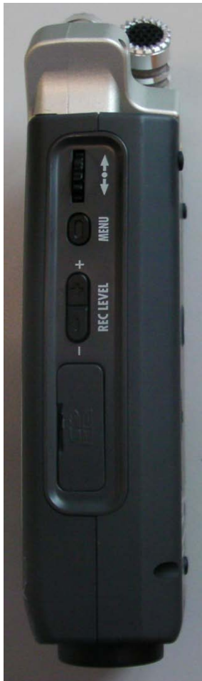
Figure 4 - Right hand spine of Zoom recorder showing the dial, button and SD flap that control the menu, recording level and enable memory card storage.
