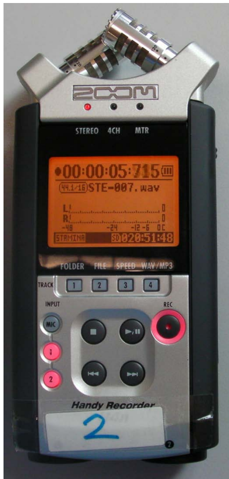
Figure 20 – When the “1” and “2” buttons are red, external microphones need to be used to capture audio.
