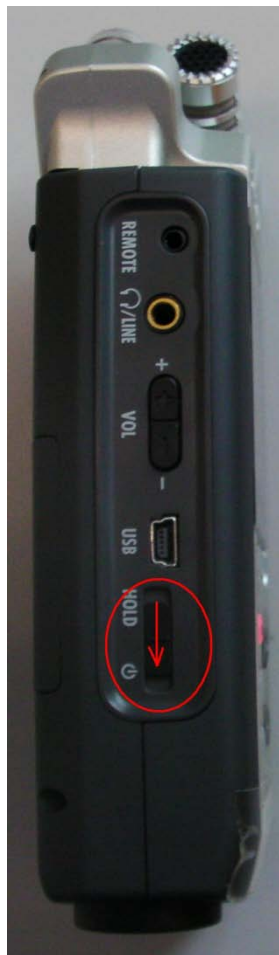
Figure 10 – The 'power on' button needs to be slid downwards and held until the display screen becomes active.
