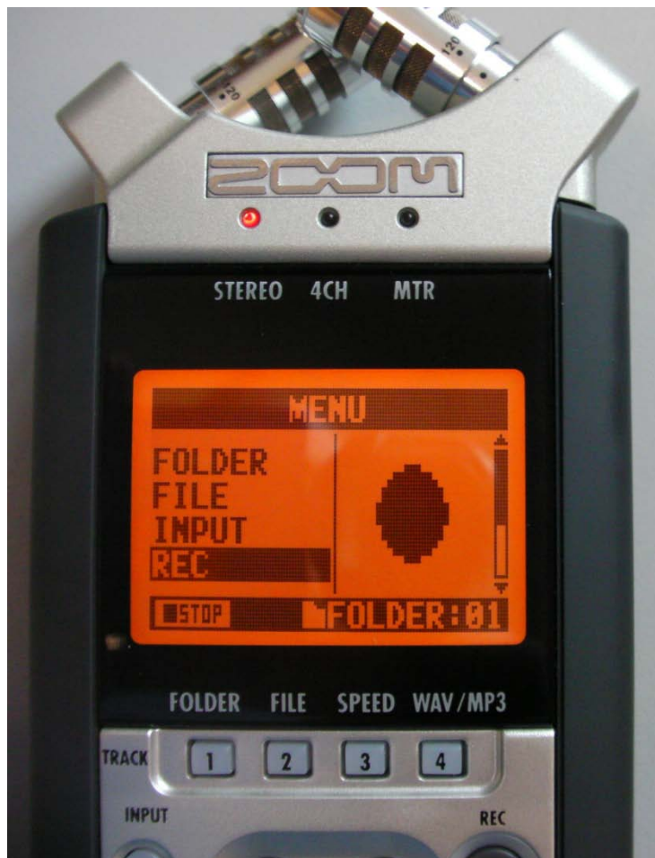
Figure 14 – The dial acts to allow scrolling in the menu and can be used to move to REC.
