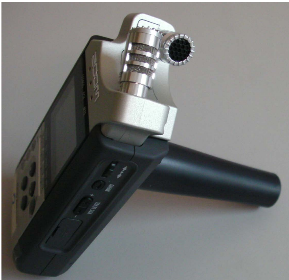
Figure 23 – Screwing the stand into the back panel of the recorder mimics a tripod.
