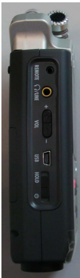
Figure 5 – Left hand spine of Zoom Recorder showing inputs for remote operation, line in, headphones and USB as well as control buttons for volume control, hold and power.
