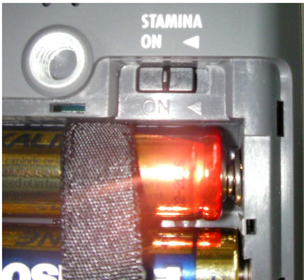
Figure 9 – Stamina mode can be selected by removing the battery cover.
