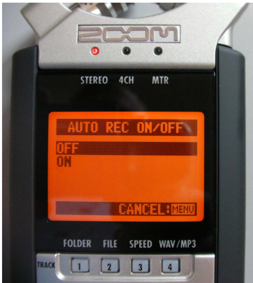
Figure 16 – Selecting the REC mode can be done by using the dial to scroll between ON and OFF.
