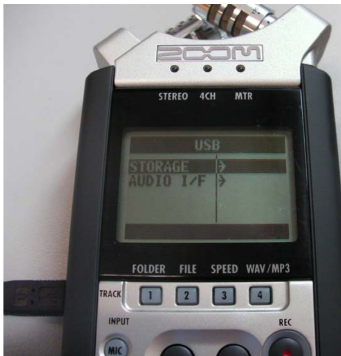
Figure 31 – Connecting a USB cable will prompt a screen showing USB.
