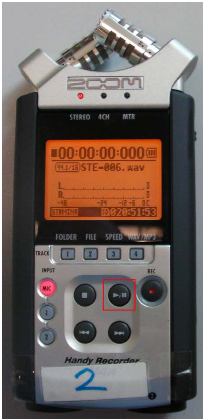
Figure 25 – The quality of the audio can be checked by pressing the play button after ending the recording.
