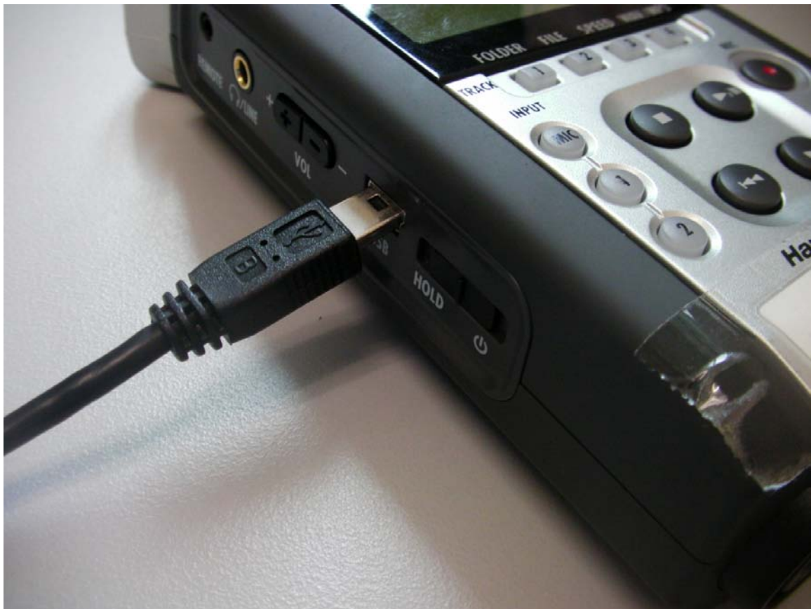
Figure 30 – Using a USB cable to connect the Zoom recorder to a computer for data transfer.
