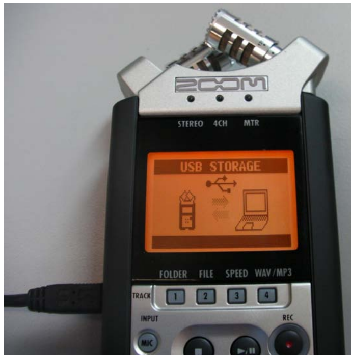
Figure 32 – Once “storage” is chosen, the Zoom recorder will connect to the computer.
