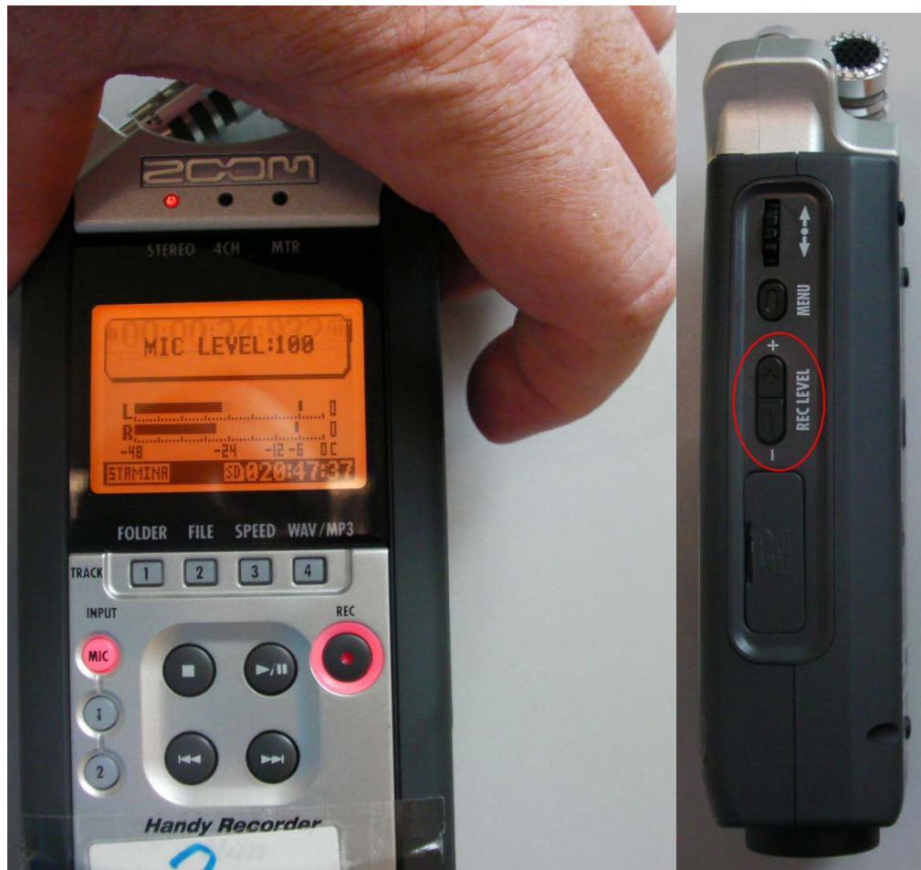
Figure 21 – The recording level can be manually adjusted when recording is underway.
