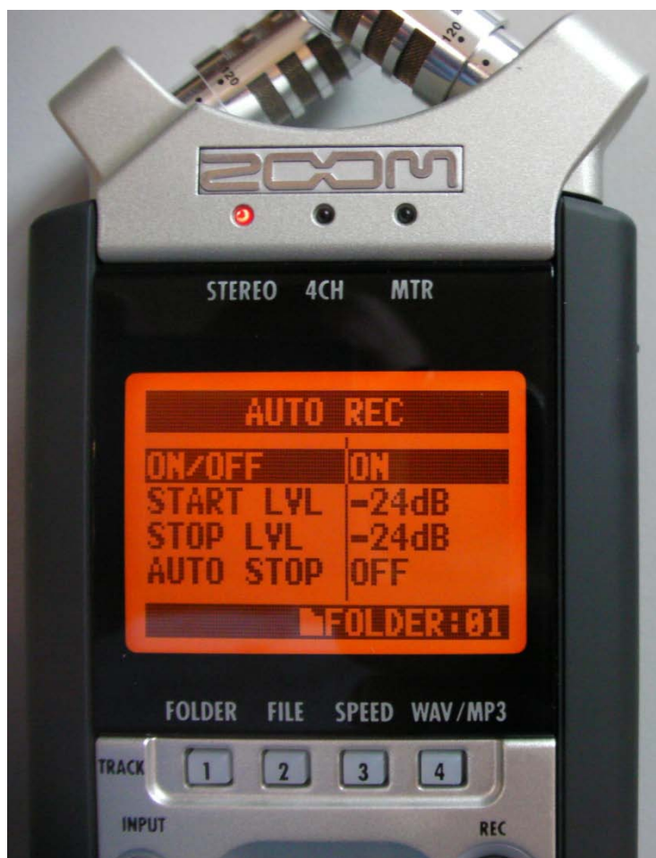
Figure 15 – The AUTO REC screen display shows it is auto recording level mode.
