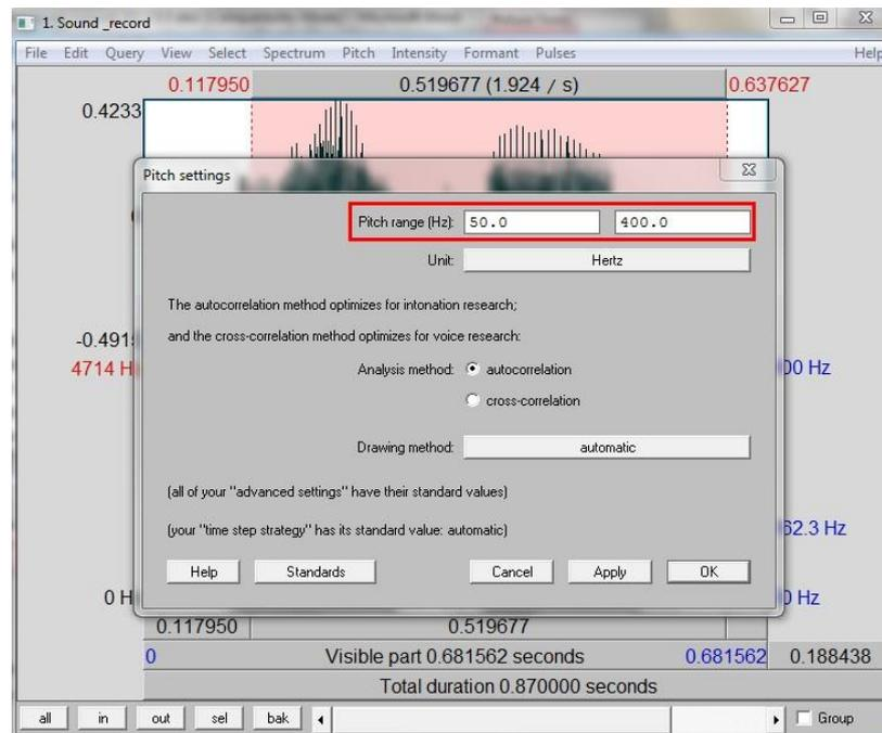
**If the pitch contour is too low in spectrogram, you can increase the maximum value of the pitch range (e.g. increase from 400 to 500); if the pitch contour is too high, you can decrease the maximum value of the pitch range (e.g. decrease from 400 to 300).**
