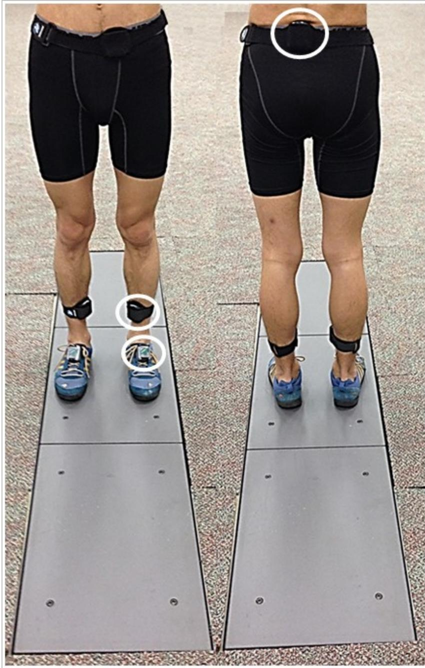
**Figure 3.2. Locations of the inertial measurement units. The foot IMUs were affixed to the instep of the shoes using flat bracelet housings and were interlaced tightly using the shoelaces. The shank IMUs were affixed to the anteromedial distal aspect of the tibiae using elastic straps. The pelvis IMU was affixed to the lumbosacral joint level using an elastic strap.**
