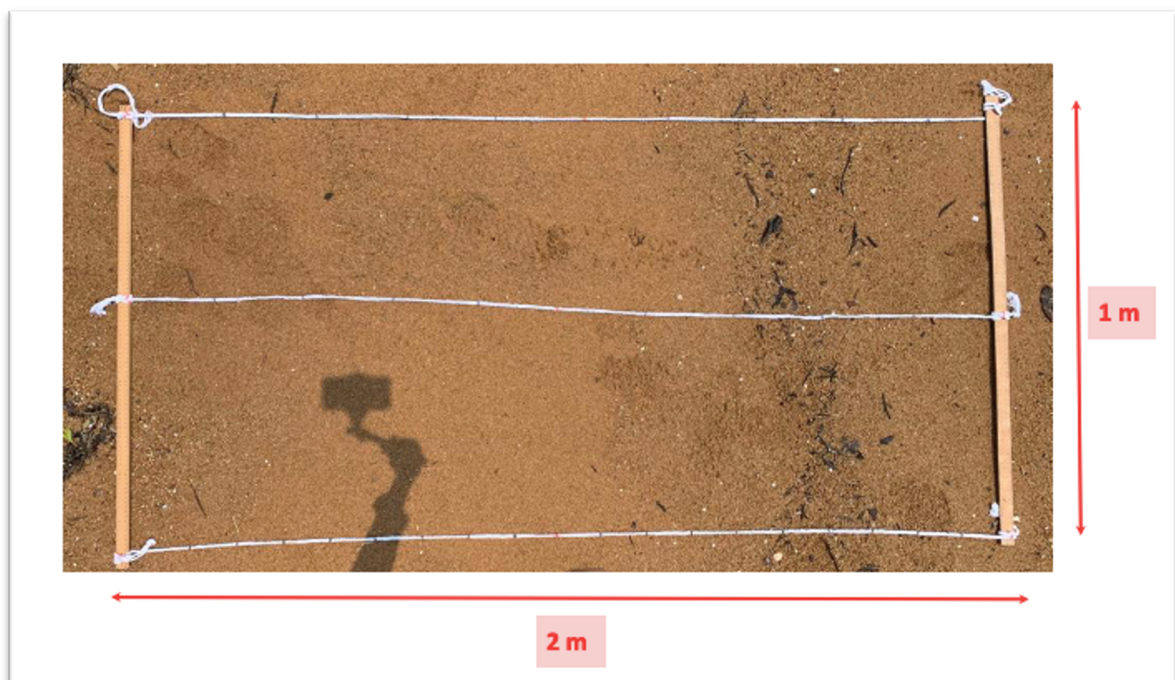
Figure 4: The sampling tool, Length:2meter, Width:1meter
