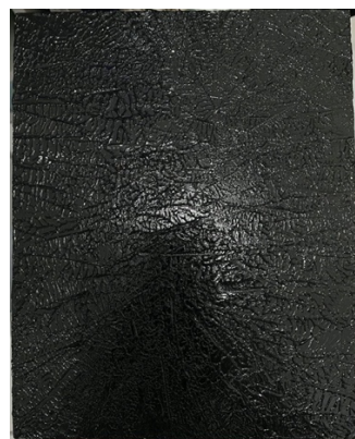
(Picture 4-10-2 Cracks before the Paints Dried)
