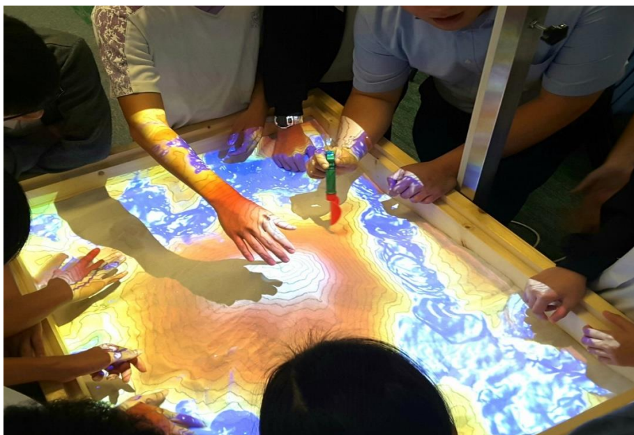
Photo 1.2 An AR Sandbox real-time augmentation on modifying topography models
