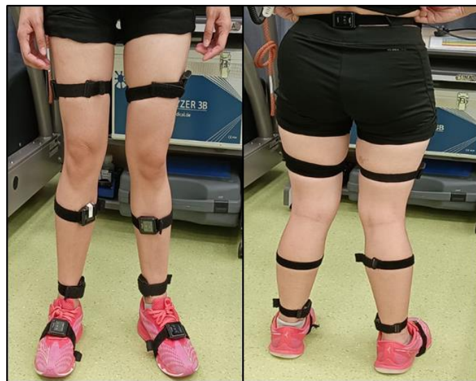
Figure 4.1: Placement of inertial measurement units on lower back at the level of L5S1 and two each on bilateral thighs, shank, and foot using elastic straps
