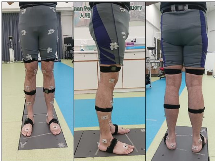
Figure 3.1: Sensor and marker positions for Opal and Vicon systems
