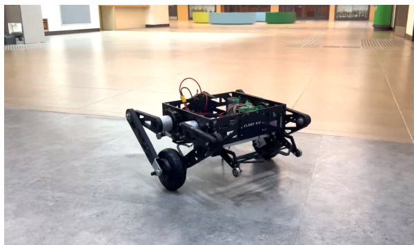
Fig. 1. Bipedal Wheeled Robot previously assembled by the researcher, showing the original platform whose concepts were translated into the EduBalancer kit.
